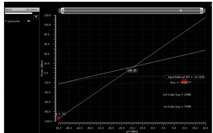
Fig 12. Simulation result of IIP3 at frf=28.5GHz & frf2=29GHz
