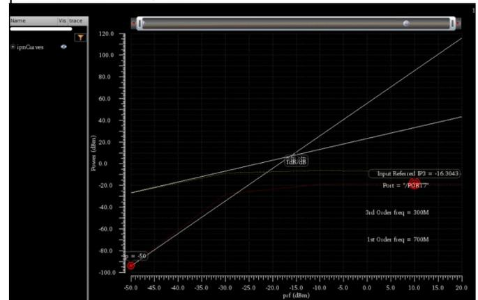
Fig 11. Simulation result of IIP3 at frf=27.5GHz & frf2=28GHz
