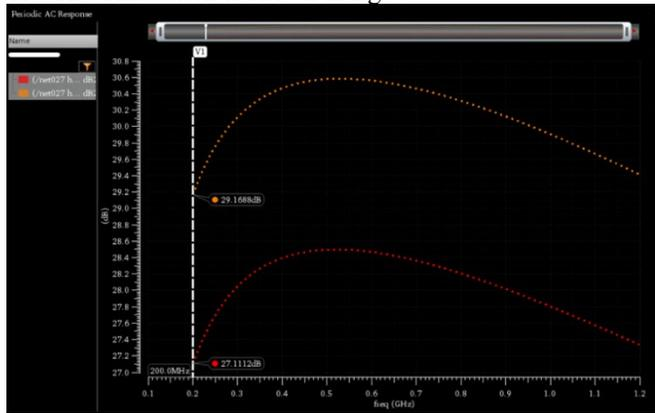
Fig 9. Simulation result of voltage conversion gain
