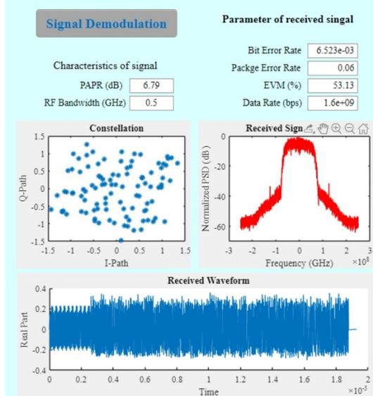
Fig 14. Simulation result of Co-simulation on EVM
