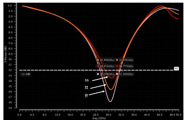
Fig 8. Simulation result of S11 [Three corner: ss & tt & ff]
