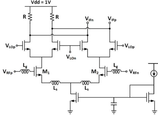
Fig 4. Proposed mixer schematic
