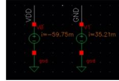
Fig 6. Current consumption at the VDD by DC analysis
