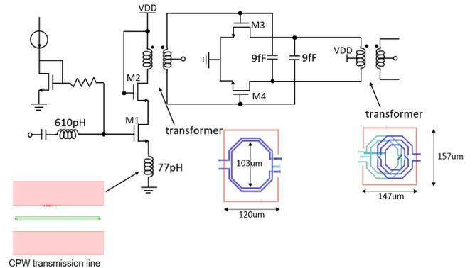
Fig 3. Proposed LNA schematic and transformer design
