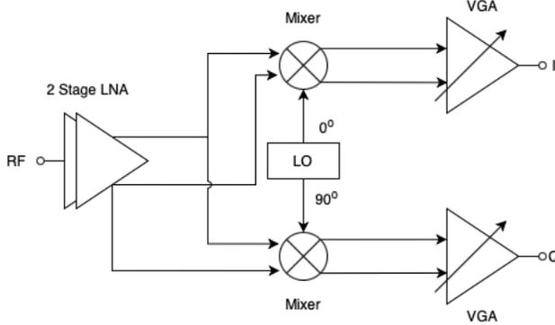
Fig 1. Proposed receiver architecture
