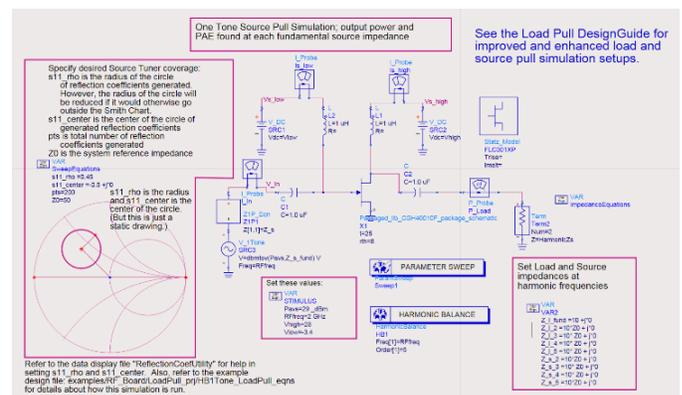
Fig. 2. Loadpull simulation setup
