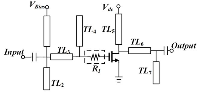
Fig. 4. Single Stage schematic of Power amplifier
