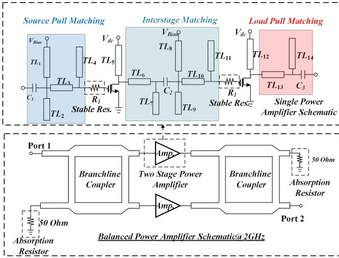
Fig. 6. Circuits diagram of the proposed power amplifier
