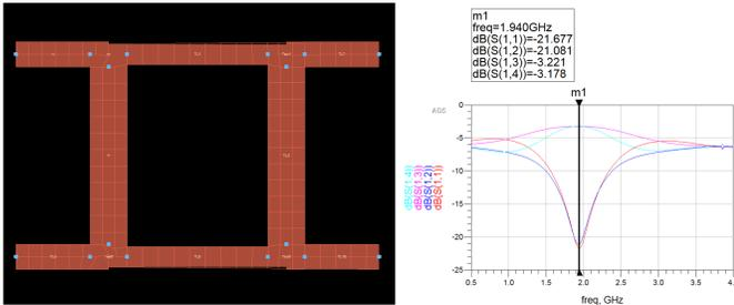
Fig. 7. Topology and simulation results of hybrid coupler
